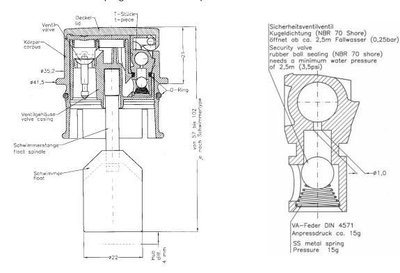
The hole inside the t-piece for the incoming water is 1mm (normally 1,5mm). A NBR-ball which will be pressed against a sealing surface by a metal spring is operating as a one way valve. The water pressure must be at least 250mbar (3,5psi) in order to open the system.
